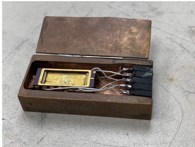
Figure D.2 : Home-made sample box for noise measurement.
